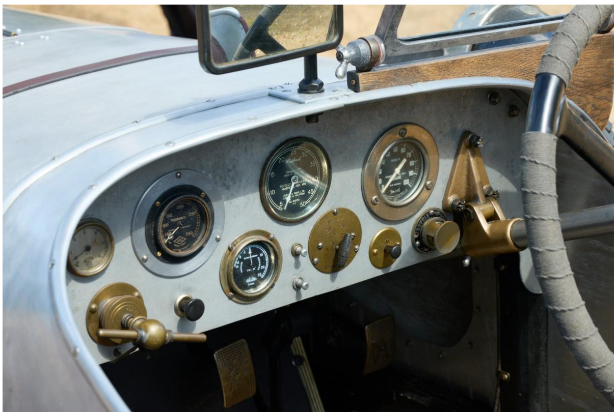
The cockpit, with supercharger boost gauge, Watford rev-counter and correct minor instruments.
