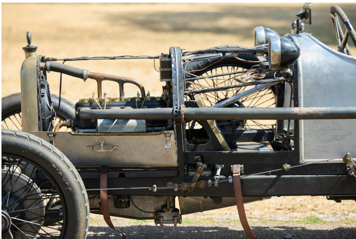
The 1½-litre side-valve engine in the chassis, built on the original crankcase of the last Works Brooklands racer.
